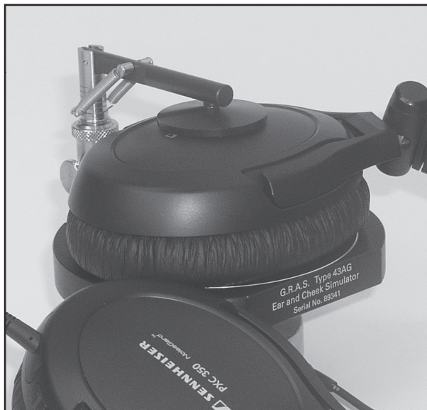
Fig. 3 Testing a headphone: The finger simulator of Fig. 2 replaced by the default-mounted disc. Both cheek simulator and clamp with disc are essential for well-defined test conditions.
