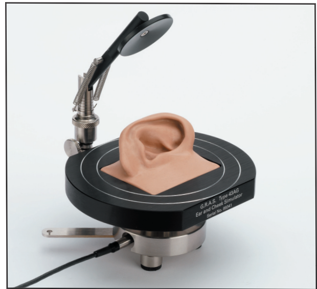
Fig. 1 Ear and Cheek Simulator Type 43AG
