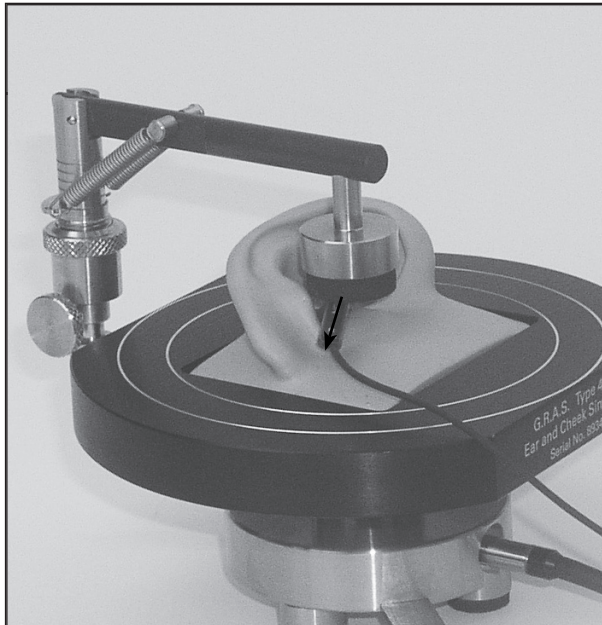
Fig. 2 Testing an earphone: The spring-loaded clamp with the finger simulator mounted allows well-defined test conditions.
