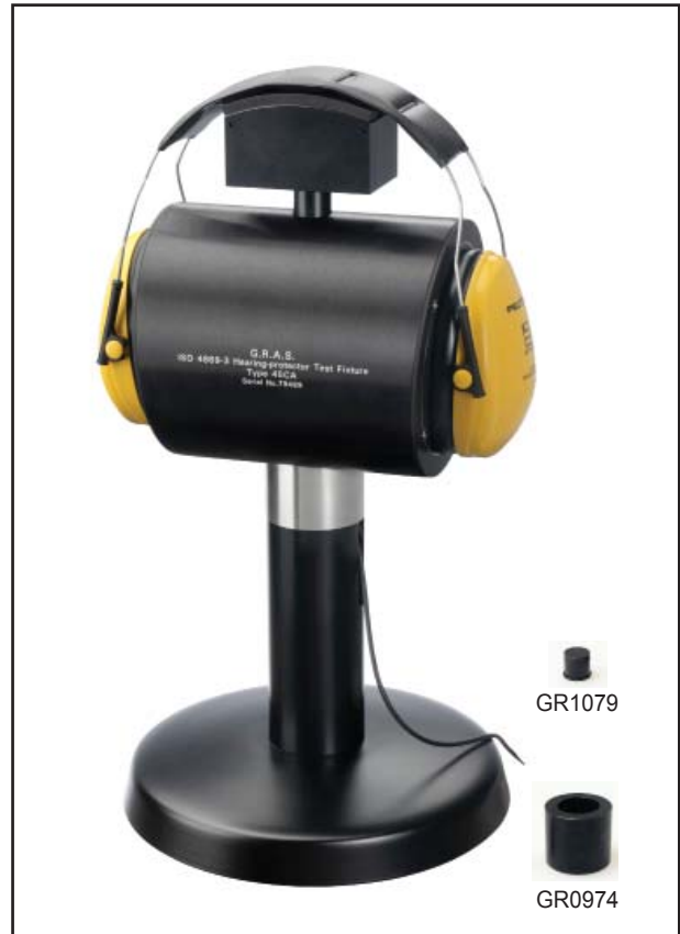
Fig. 1 Hearing-protector Test Fixture Type 45CA. On the right: Blind Plug GR1079 and Cup GR0974.
