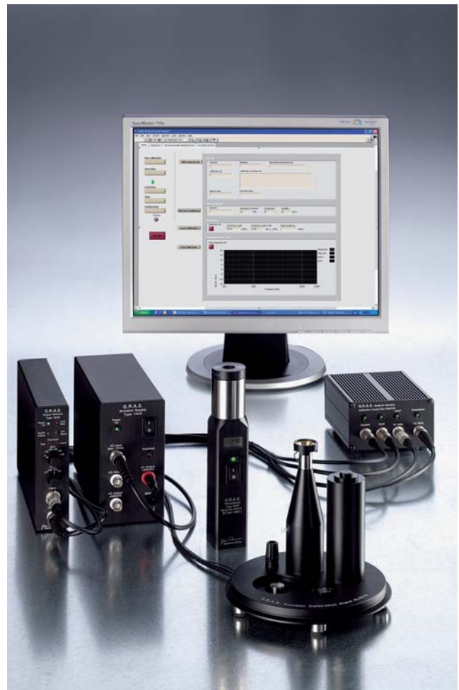
Fig. 1 A typical setup for the Microphone Calibration System 90CA
